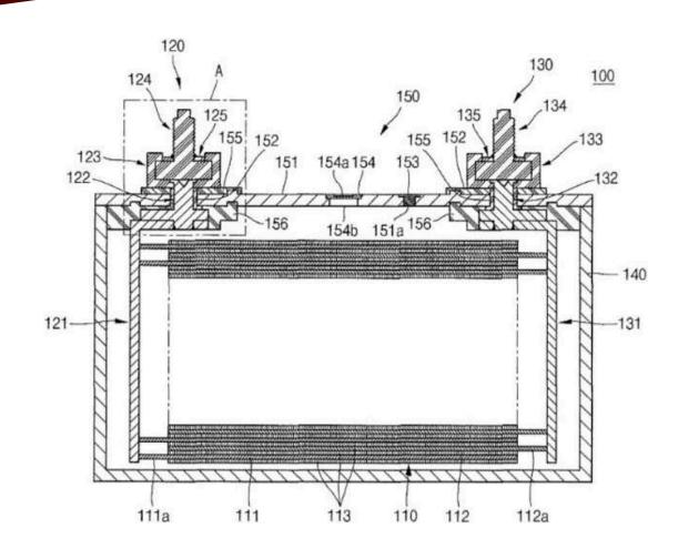
▶ Body not in contact with the positive electrode: Some designs included gaskets on either on the upper section or lower section, but not both, missing the dual-gasket arrangement.
